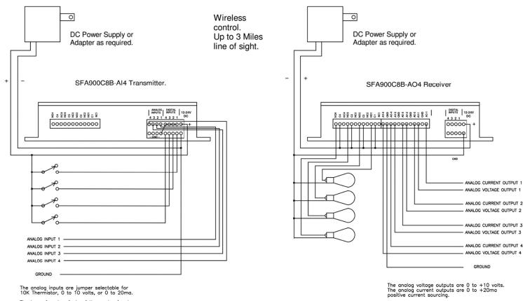
The analog inputs are jumper selectable for 10K Thermistor, 0 to 10 volts, or 0 to 20ma.
