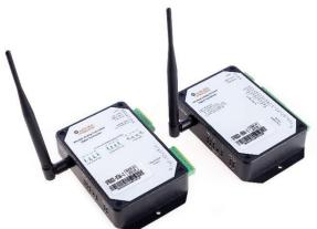
These products utilize spread spectrum technology and are immune to interference and multipath fading. These systems will not interfere with wifi networks.
