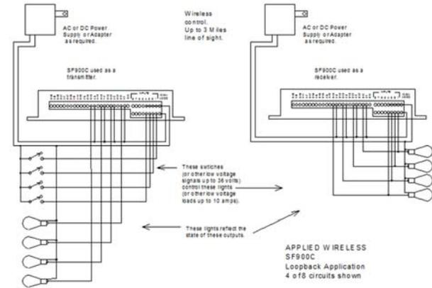
In loopback mode, the relay is activated as in the earlier example. However, in Loopback mode, a transmission will then be sent back to the originating location and a relay activated as feedback that the remote operation has been carried out.
